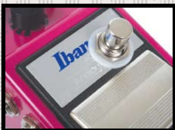
■ The Keeley Ibanez AD9 is fitted with a true-bypass switch and upgraded components
